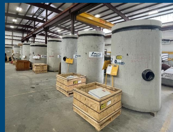
Pump Lift Stations
