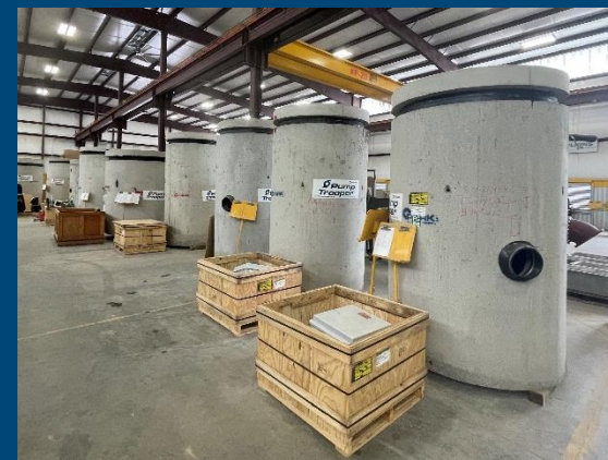
Pump Lift Stations
